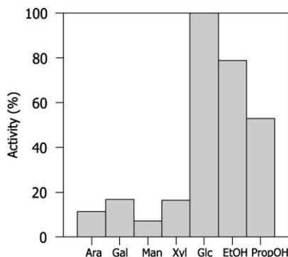
Fig. 1. Response of *Gluconobacter oxydans* microbial biosensor to various substrates. The cells were cultivated on L-arabitol as a sole carbon source at 28°C. Legend: 100% is the response to D-glucose. Ara: arabinose; Gal: galactose; Man: mannose; Xyl: xylose; Glc: glucose; EtOH: ethanol; PropOH: propanol.
