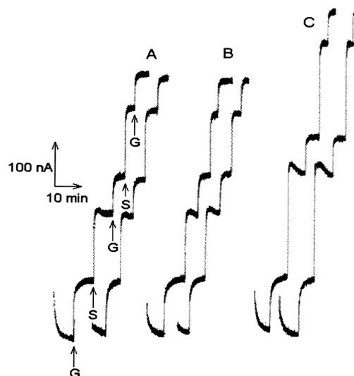
Fig. 6. Record of duplicate standard–sample–standard–sample–standard assays of three samples. A: sample 3 ( $50 \mu\text{l}$ ); B: sample 4 ( $20 \mu\text{l}$ ); and C: sample 5 ( $20 \mu\text{l}$ ). Measurements were carried out before evaporation of ethanol and propanol, using  $200 \mu\text{l}$  of a  $1 \text{ g l}^{-1}$  glucose solution. G: standard glucose solution, S: sample of lignocellulose hydrolysate.
