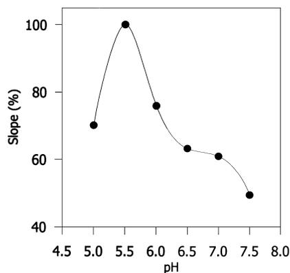
Fig. 2. Effect of pH on microbial biosensor response; 100% is the maximum response, as in the following figures. Measured in phosphate buffer at 30°C, at a working potential of +300 mV and with 3 mM hexacyanoferrate(III).
