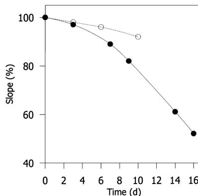
Fig. 5. Storage stability of the biosensor. Biosensors were stored at 4°C in the dry state (●), and in phosphate buffer pH 5.5 (□); 100% is the biosensor response determined on the first day.
