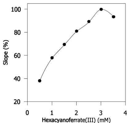
Fig. 4. Effect of mediator concentration on the biosensor response. For other conditions used see Fig. 2.
