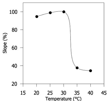
Fig. 3. Effect of temperature on biosensor response. Measurements were done in phosphate buffer at pH 5.5. Other conditions as in Fig. 2.
